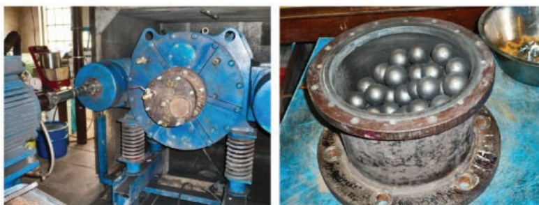
Fig. 1. Eccentric vibratory mill with attached closed satellite (left), open satellite filled with balls (right) (Baláž 2018)
