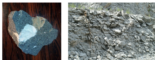
Fig. 9. Natrolitic trachyte, mined by the quarry in Mariánská skála; fracturing of the rock as a result of stress relief during the outcrop of the massif (laccolith) during Saxon tectogenesis
