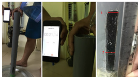
Fig. 8. Experiment for determining the water separation of backfill materials
