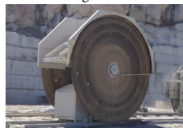
Fig. 10. Disc sawing machine at the quarry.
