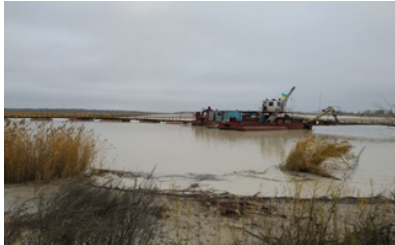
Fig. 7. Development of man-made deposit of titanium-zirconium ores by hydromechanized method
