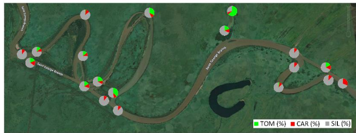
Fig. 2. The spatial distribution of the main lithological components (TOM%, CAR%, SIL%) in bed sediments:
