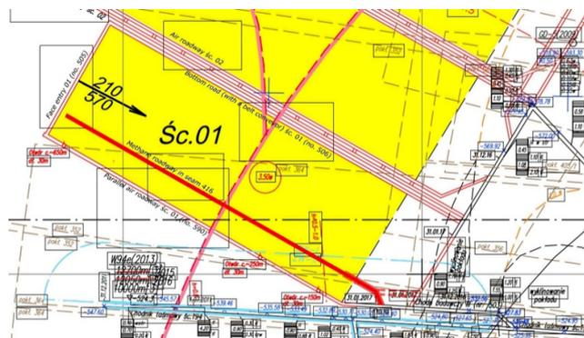
Fig. 3. Drainage roadway location behind the longwall panel
