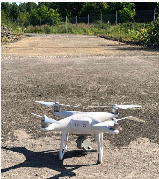
Fig. 2. a) Preparing the drone for measurement - before applying the mineral-asphalt mixture, b) measurement of control points using GNSS satellite technology.
