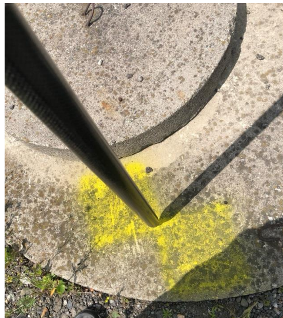
Fig. 2. a) Preparing the drone for measurement - before applying the mineral-asphalt mixture, b) measurement of control points using GNSS satellite technology.
