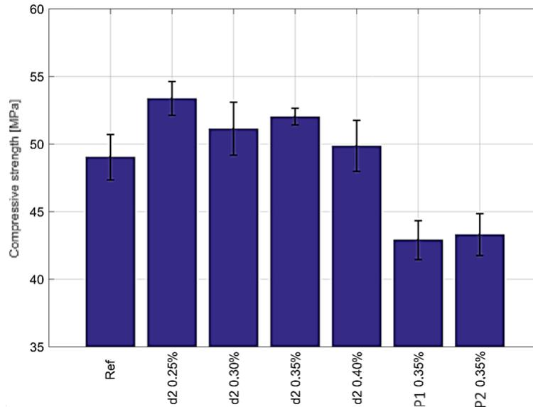
Fig. 3. Compressive strength of cement mortar beams with dextrin admixtures d2.
