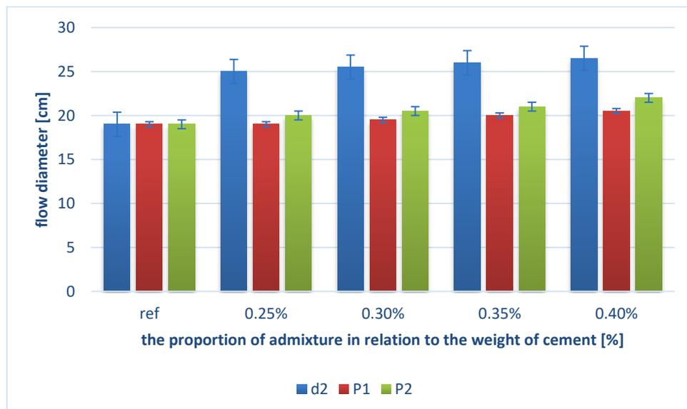
Fig. 2. Flow diameters of mortar cement with admixture d2 and plasticizers P1 and P2.
