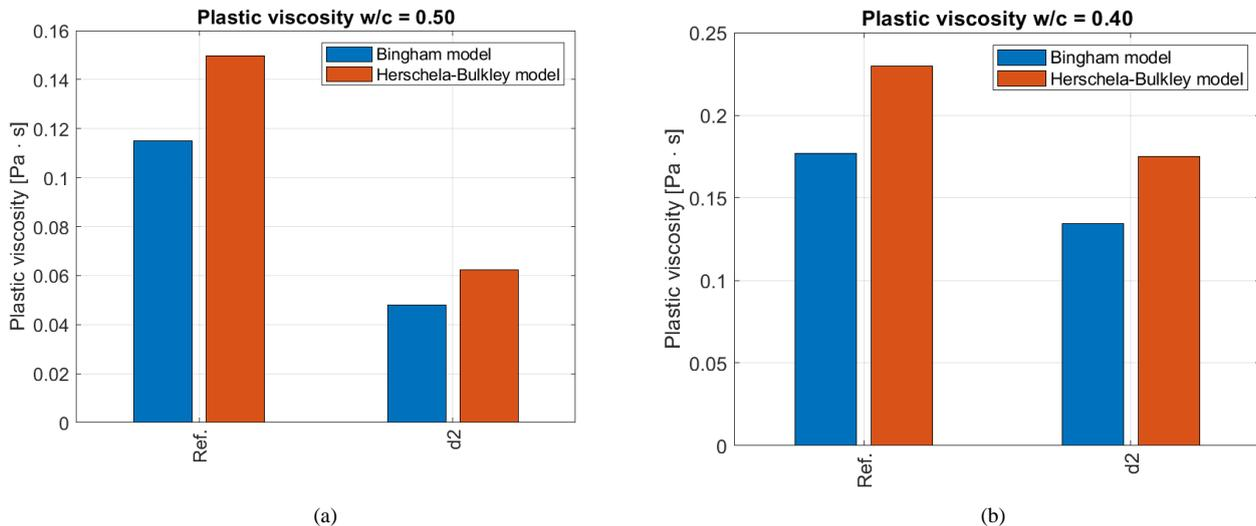
Fig. 4. Plastic viscosity of cement slurries for w/c = 0.50 (a) and w/c = 0.40 (b).
