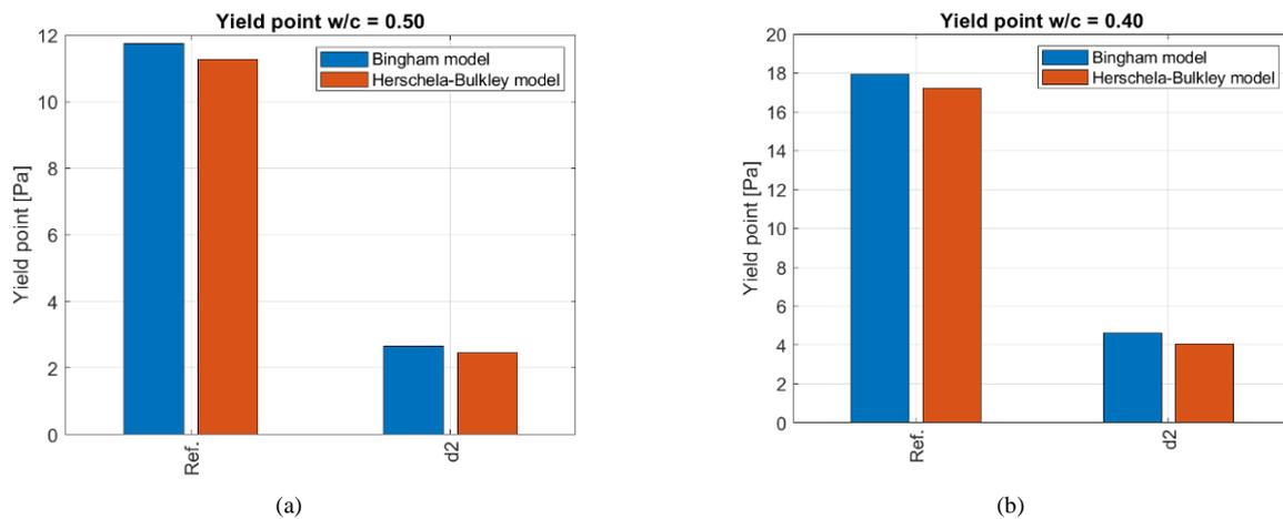
Fig. 5. Yield point of cement slurries for w/c = 0.50 (a) and w/c = 0.40 (b).
