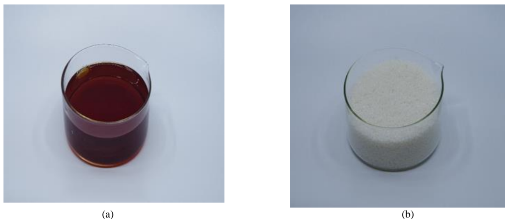
Fig. 1. Chemical additives used for foaming of asphalt 50/70: surface active substance (a) and synthetic wax F-TLC (b).
