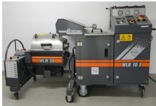
Fig. 2. WLB-10S test stand for the production of foamed asphalt [21]
