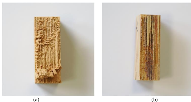
Fig. 10. Representation of the shear zone of the “Length”-specimens, (a) bamboo failure, and (b) bamboo and glue line failure.
