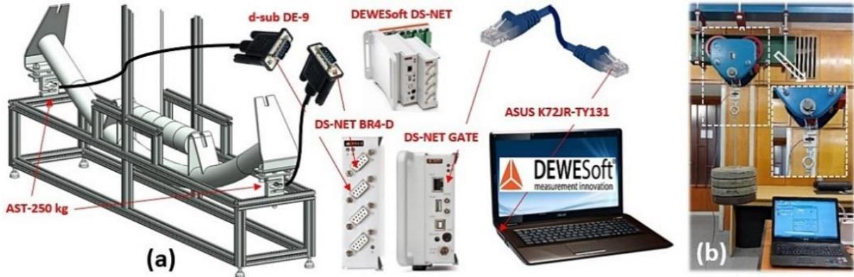
Fig. 3. (a) measuring chain of laboratory equipment, (b) calibration of strain gauge force sensors with weights of a known mass.
