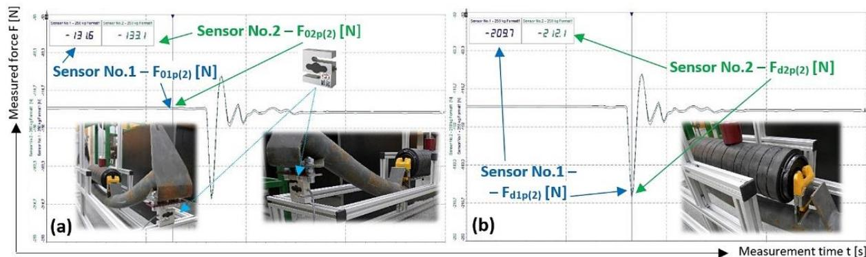
Fig. 7. Recording of measured forces (a)  $F_{01p(2)}$  [N] and  $F_{d1p(2)}$  [N] taken by the force sensor No. 1, (b)  $F_{02p(2)}$  [N] and  $F_{d2p(2)}$  [N] by force sensor No. 2.
