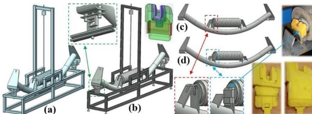
Fig. 2. Laboratory equipment (a) welded frame, (b) bolted frame, (c) standard troughing idler, (d) impact troughing idler.
