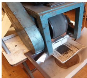
Fig. 3. Magnetic separator – reception of diamagnetic material [own elaboration]
