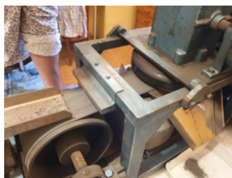
Fig. 2. Magnetic separator – vibrating material feeder [own elaboration]
