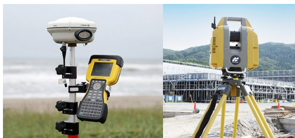
Fig. 1. Modern GNSS and TLS equipments. Source: (left) https://ts-geosystems.com/product/trimble-r8-rtk-gps/ and (right) https://ajhsurveyors.com/wp-content/uploads/2020/11/2-3.jpg
