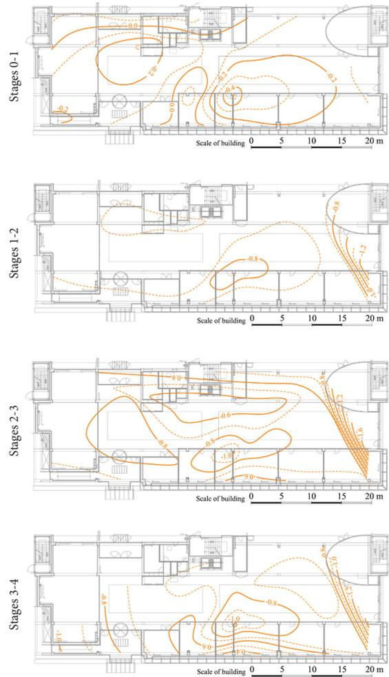
Fig. 7. Graphical visualization of height changes between neighbouring stages of geodetic measurement
