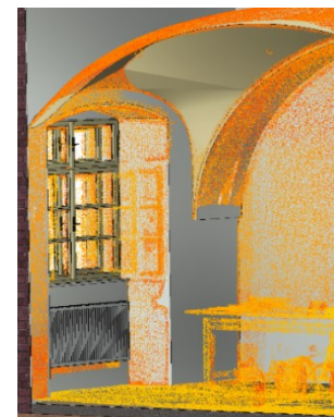
Fig. 4c. Deviation of the point cloud from the model (view)
