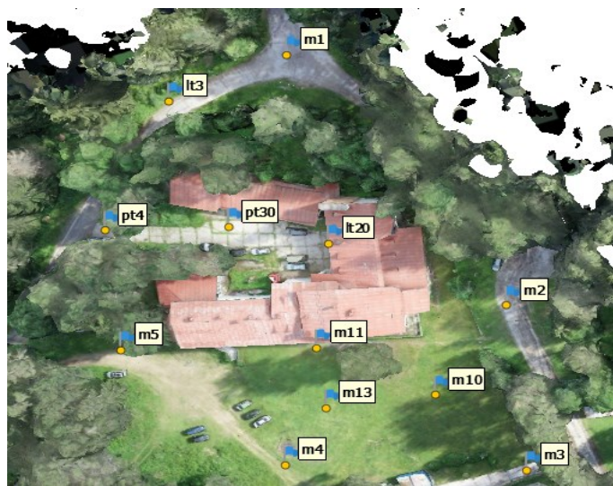
Fig. 2. Scheme with the location of the GCP
