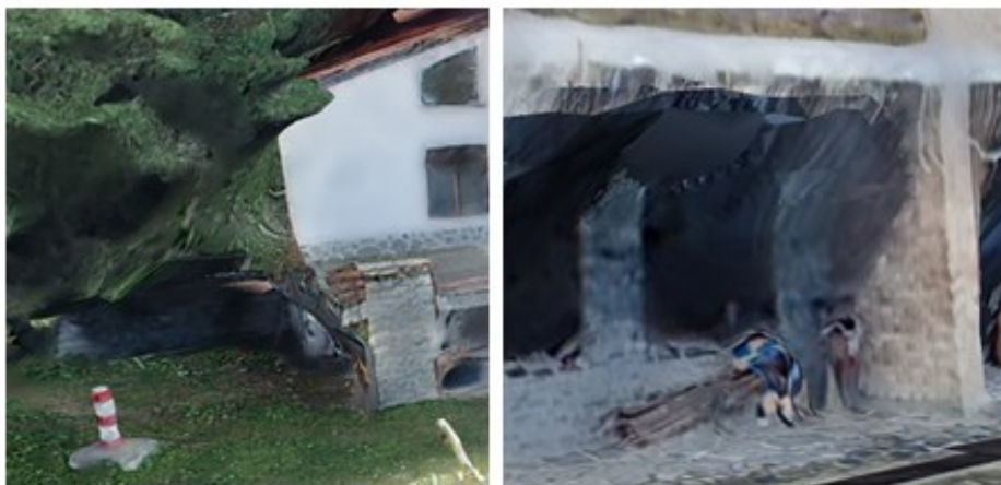
Fig. 11. Disadvantages of 3D models obtained by aerial photography with a UAV
