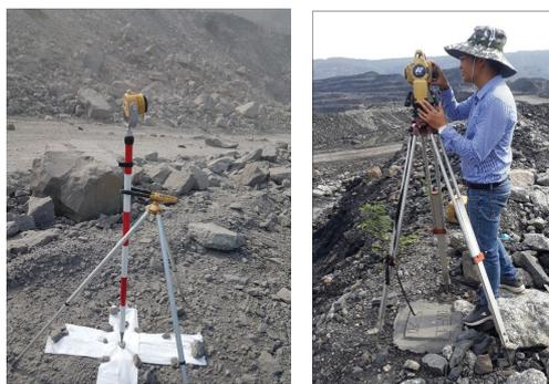
Fig. 6. An example of a GCP on the test site and measurement by a total station
