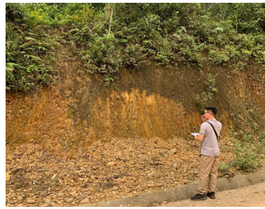
Fig. 7. Deformed limestone (right) and claystone steep dipping in Moc Chau-Tam Diep milonite fractured zone
