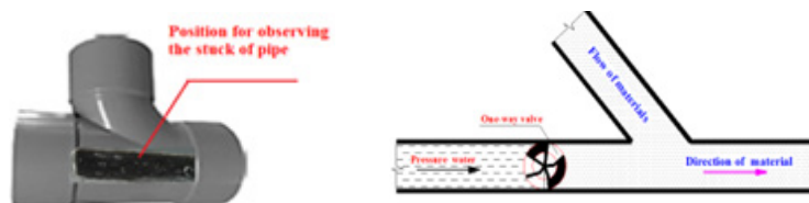
Fig. 5. Diagram of layout the points changing the flowing direction
