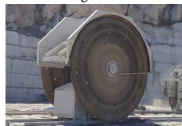
Fig. 10. Disc sawing machine at the quarry.
