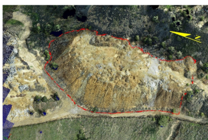
Fig. 3. Digitisation of the stockpile boundary on the point cloud dataset [48]
