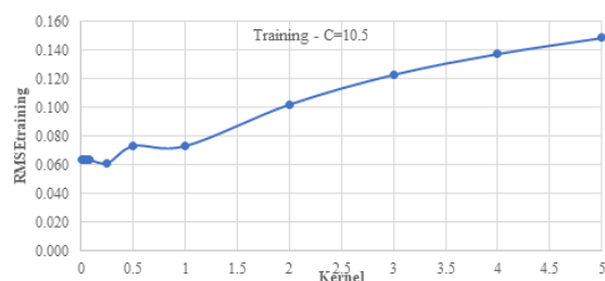
Fig. 6. The graph shows the dependence of the RMSE on the Kernel scale in the training dataset of the optimum SVR model
