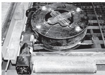
Fig. 1. Device for rotating with sample under the AWJ cutting head
